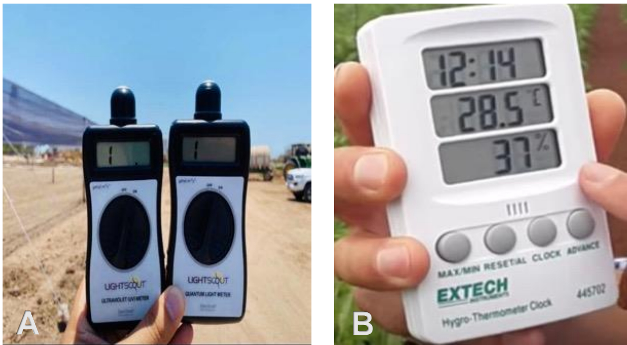
Figura 8. A) Sensores LIGHTSCOUT Ultraviolet Meter y LIGHTSCOUT Light Meter Quantum, e inciso B) Higrómetro Extech.
